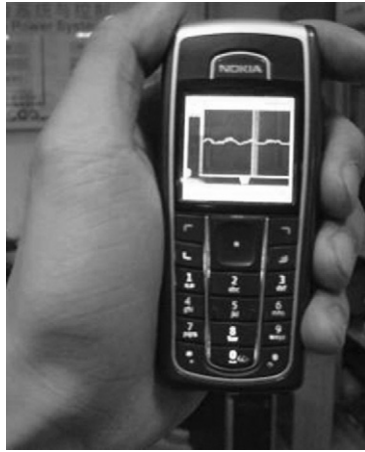
Fig. 11. Fuel cell bus status on-line monitoring on cell phone.
